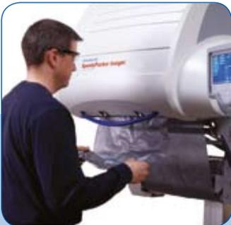
1. With the push of a button, the SpeedyPacker® Insight™ system quickly dispenses an Instapak® foam-filled bag.
