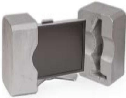
The Instamoulder™ system can produce up to 600 protective cushions an hour, ideal for high-volume operations. The unit comes in 8, 10 or 12 mould box configurations and only requires 4 m<sup>2</sup> of floor space.
