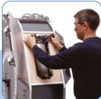
2. When placed into the mould enclosure, the bag is drawn in by an on-board vacuum.
