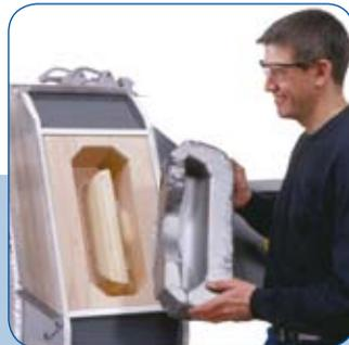
3. After the cushion has fully expanded, it is removed with the help of a built-in air ejection system.
